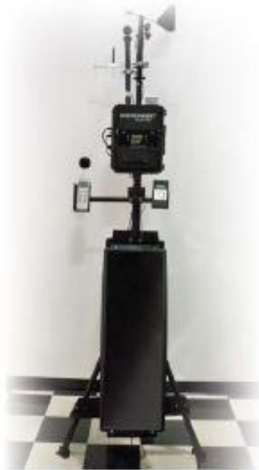
HAZ-SCANNER EPAS shown with optional solar panel
