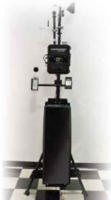
HAZ-SCANNER EPAS shown with optional solar panels
